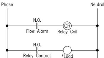
\* The load must be within the Flow Alarm's contact rating. Please see specifications.
