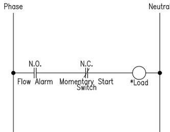
\* The load must be within the Flow Alarm's contact rating. Please see specifications.
