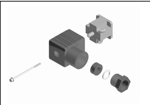
of a screwdriver into the slot marked for that purpose. Illustration 6 shows the disassembled female section.
