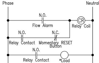
\* The load must be within the Flow Alarm's contact rating. Please see specifications.
