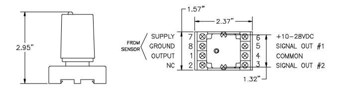
The module is built into a casing which plugs into an 8 pin octal style base. Wiring connections are made to the base which can be mounted by panel screws or using a DIN rail mount. To access the signal jumpers, J1 and J2, remove the casing from the octal base, then remove 4 screws to separate the case.
