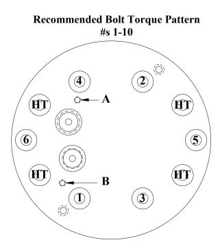
Holes Labeled "HT" = Hand Tight Holes labeled "A" & "B" are sensor bracket **mounting holes.**
