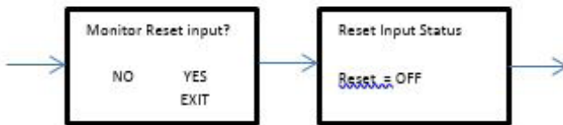
Figure 34. Monitoring External Reset Input
