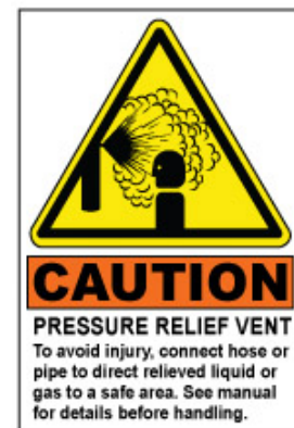
Fig. 3: Warning sticker found near the rupture disc on all meters
