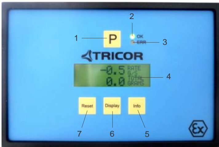
Fig. 2: Operating Elements of TCE 8***-L*-Ex
