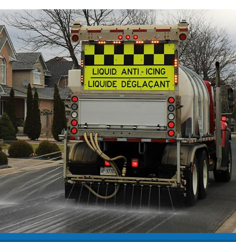
**APPLICATION SPOTLIGHT** Chemical Spraying – Anti-Icing & De-Icing Vehicles
