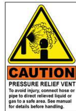
Fig. 2: Warning label near the bursting disc
