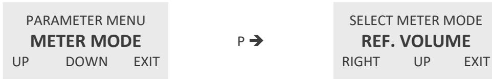
After confirming with “P”, you will be asked to make the settings required for the gas measuring mode.
