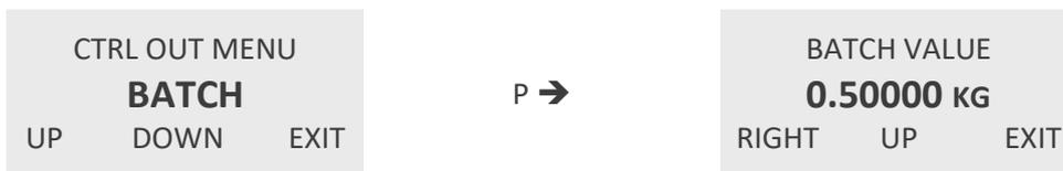
Use the keys "RIGHT" and "UP" to select the desired step value and confirm with "P" or skip with "EXIT".
