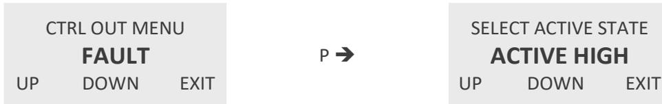
Use the keys "UP" and "DOWN" to select the desired value and confirm with "P" or skip with "EXIT".
