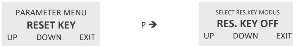
Use the keys “UP” and “DOWN” to enable or disable the key and confirm with “P” or skip with “EXIT”.
