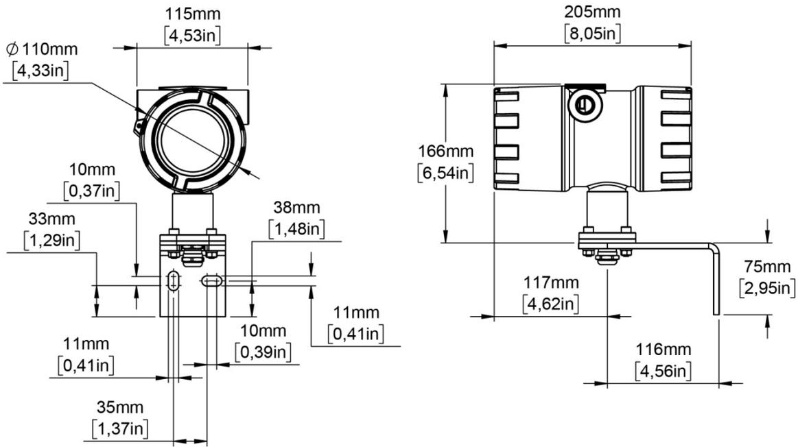
Fig. 39: Dimensions Wall-Mount Transmitter TCE 8000/8100 (for hazardous area)
