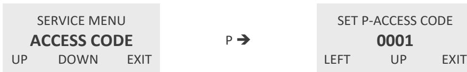
Change the indicated number with “LEFT” and “UP” to the desired code number and confirm with “P”.
