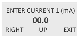
Use the keys “RIGHT” and “UP” to select the desired value and confirm with “P” or skip with “EXIT”.
