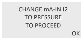
Confirm with “OK”. Configure the analog input correspondingly (see chapter 4.5.8.5) and repeat the setting.
