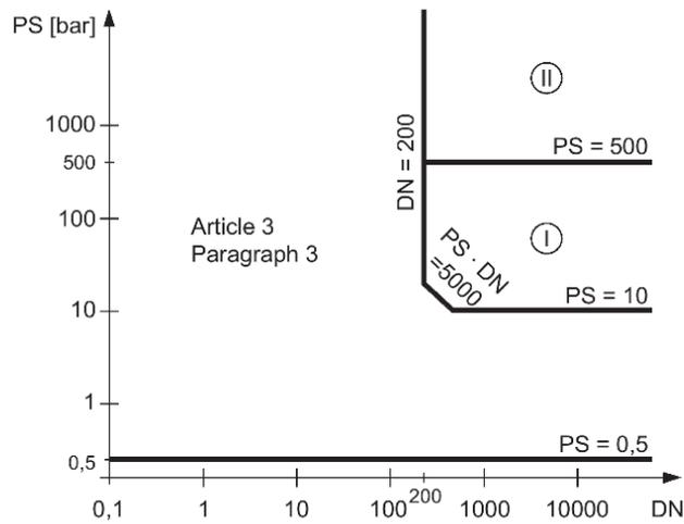
Fig. 28: Diagram 2 for gases of fluid group 2
