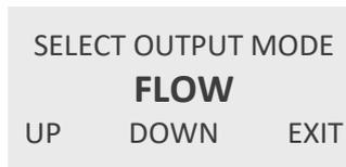
Use the keys “UP” and “DOWN” to select the desired output value and confirm with “P” or skip with “EXIT”.
