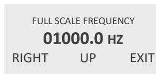
Use the keys "RIGHT" and "UP" to select the desired frequency and confirm with "P" or skip with "EXIT".
