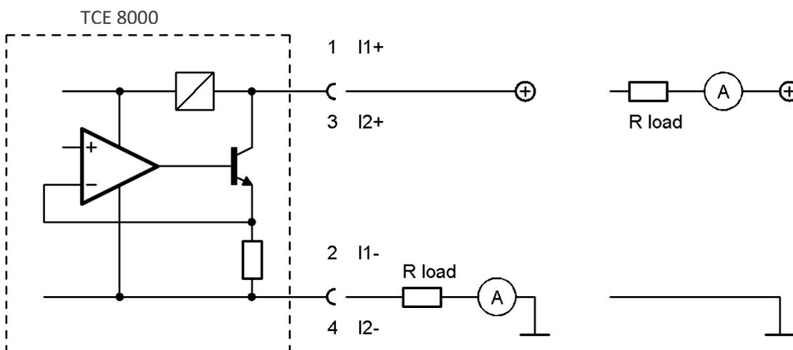
Fig. 23: Wiring diagram for 4 ... 20 mA current loop
