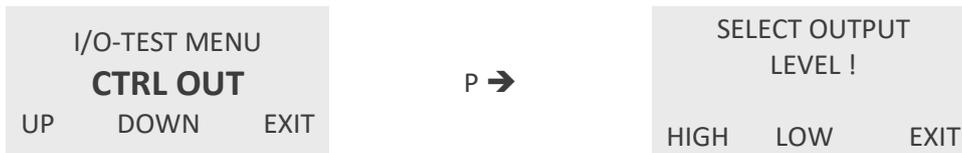
Use the keys “HIGH” and “LOW” to set the output value or leave the menu with “EXIT”.
