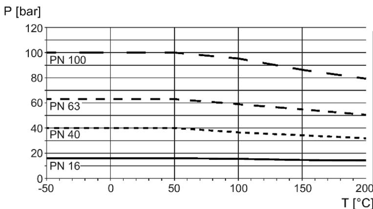
Fig. 29: Metric flange ratings, EN 1092-1 (previously DIN 2628, DIN2629, DIN 2635, DIN 2636, DIN 2637, DIN 2638)
