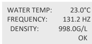
Confirm with “OK”. The display returns to the “WATER CALIBRATION” menu.
