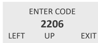
Change the indicated number with “LEFT” and “UP” to “2207” and confirm with “P”. If a wrong code is entered, the display shows “ERROR” for about two seconds and then asks for a new input.
