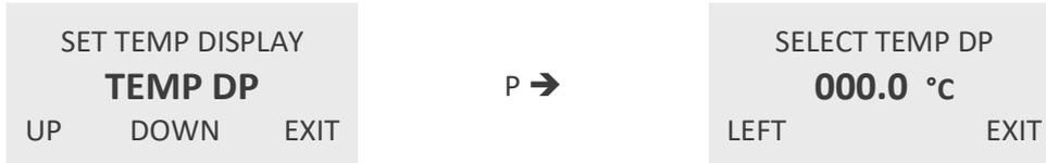
Use the key “LEFT” to select the desired decimal point position and confirm with “P” or skip with “EXIT”.
