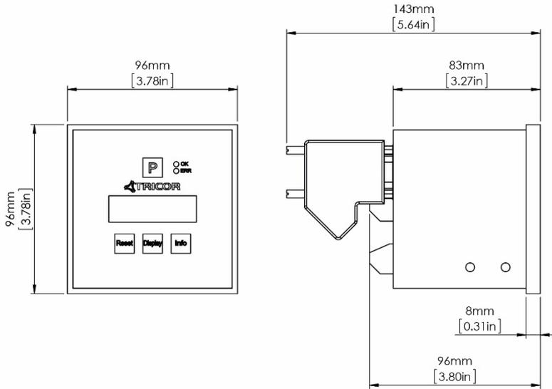
The required cutout for the panel is 92 mm +0.8/-0 mm x 92 mm +0.8/-0 mm.
