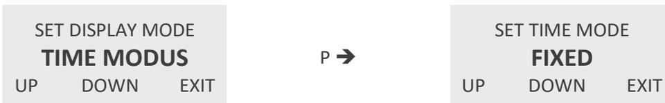
In the “FIXED” mode the display shows constantly the defined display view 1 or 2. With the pushbutton “DISPLAY” it is possible to switch over between display view 1 or 2.
