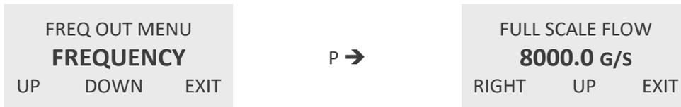
Use the keys "RIGHT" and "UP" to select the desired full scale value and confirm with "P" or skip with "EXIT".
