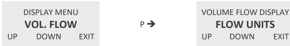
Use the keys “UP” and “DOWN” to select the submenu and confirm with “P” or skip with “EXIT”.
