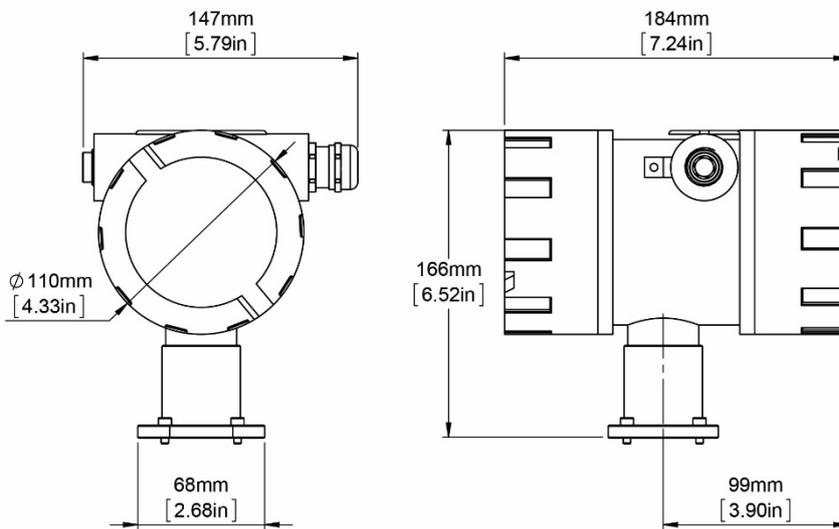
Fig. 40: Dimensions Meter-Mount Transmitter TCE 8000/8100 with blind cover
