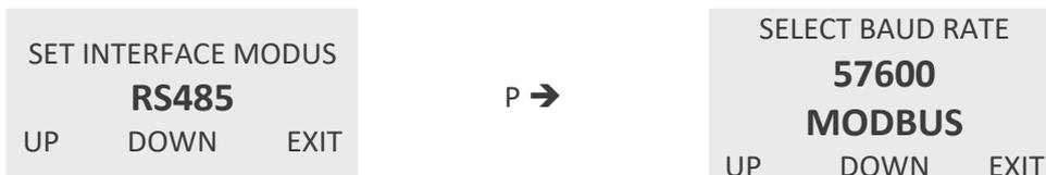
Use the keys "UP" and "DOWN" to select the baud rate and confirm with "P" or skip with "EXIT".
