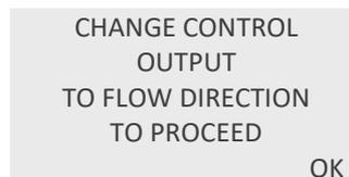
Confirm with "OK", configure the control output correspondingly, (see chapter 4.5.8.2) and repeat the setting.
