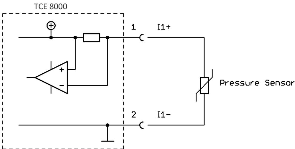
Fig. 24: Wiring diagram for 4 ... 20 mA current input
