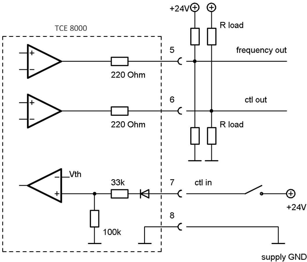
Fig. 22: Wiring diagram for digital I/O connections
