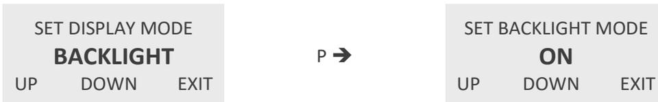
Use the keys “UP” and “DOWN” to switch on or off the backlight and confirm with “P” or skip with “EXIT”.
