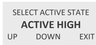
Use the keys “UP” and “DOWN” to select the desired value and confirm with “P” or skip with “EXIT”.
