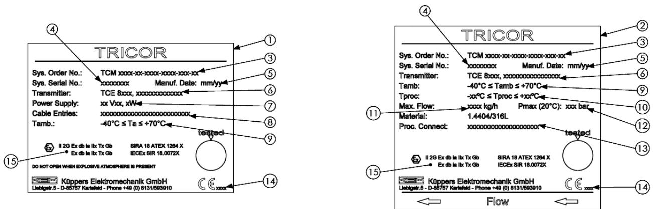
Fig. 14: Device marking TCM compact version
