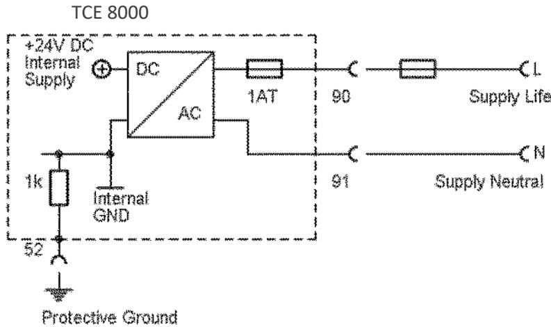
Fig. 21: Wiring diagram for power connections, AC operation
