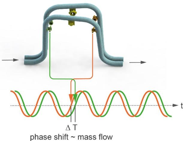
Fig. 5: Principle of operation Coriolis Mass Flow Meter
