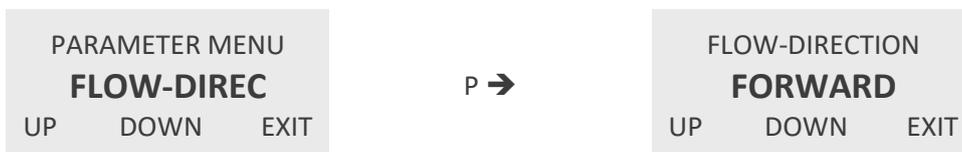
Use the keys “UP” and “DOWN” to select the positive flow direction and confirm with “P” or skip with “EXIT”.
