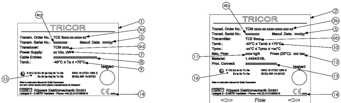
Fig. 15: Device marking TCM remote version
