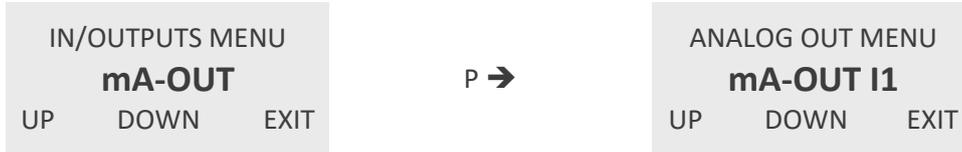
Use the keys “UP” and “DOWN” to select the desired output channel and confirm with “P” or skip with “EXIT”. The standard TCE electronics provides two analog 4 ... 20 mA outputs, I1 and I2. If the option “PRESSURE COMPENSATION” is installed, only the output I2 is available.
