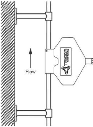
Fig. 17: Vertical Installation
