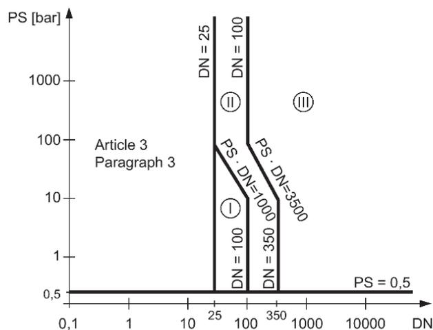
Fig. 25: Diagram 1 for gases of fluid group 1
