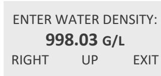
Use the keys “RIGHT” and “UP” to set the reference density and confirm with “P” or skip with “EXIT”.
