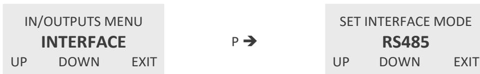
Use the keys "UP" and "DOWN" to select the desired mode and confirm with "P" or skip with "EXIT".
