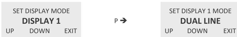
Use the keys “UP” and “DOWN” to select dual line or single line and confirm with “P” or skip with “EXIT”.
