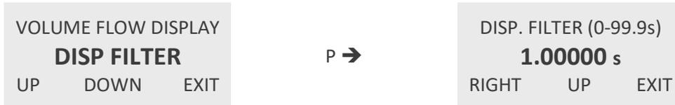
The time constant  $t$  is the time the displayed value needs after a jump from a value  $x$  to 0 to go to  $x/e = x/2.72$ .
