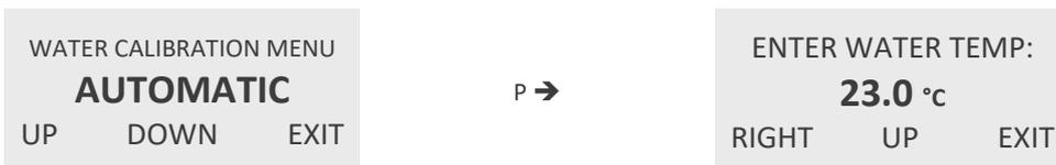
Use the keys “RIGHT” and “UP” to set the reference temperature and confirm with “P” or skip with “EXIT”.
