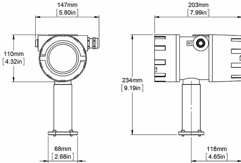
Fig. 41: Dimensions Meter-Mount Transmitter TCE 8000/8100 High Temperature
