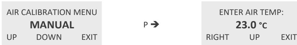
Use the keys “RIGHT” and “UP” to set the reference temperature and confirm with “P” or skip with “EXIT”. The display shows:
