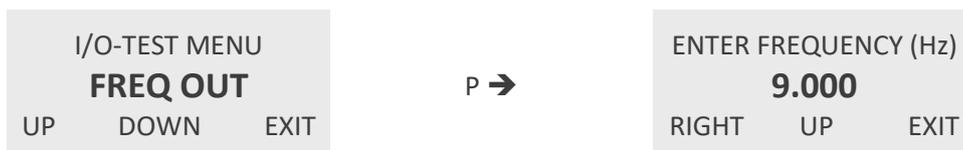
Use the keys “RIGHT” and “UP” to select the desired value and confirm with “P” or skip with “EXIT”.
