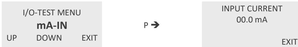
After evaluating the input, press “EXIT” to return to the “SETUP - I/O-TEST” menu.
