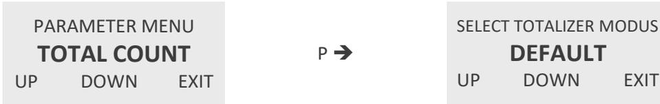
Use the keys “UP” and “DOWN” to select the mode and confirm with “P” or skip with “EXIT”.
