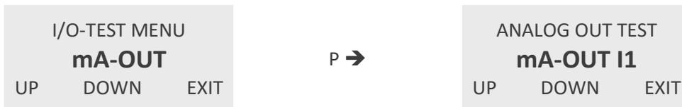
Use the keys “UP” and “DOWN” to select the desired output and confirm with “P” or skip with “EXIT”.
