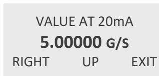
Use the keys “RIGHT” and “UP” to select the desired value for 20 mA and confirm with “P” or skip with “EXIT”. The display returns to the “SETUP - IN/OUTPUTS” menu.
