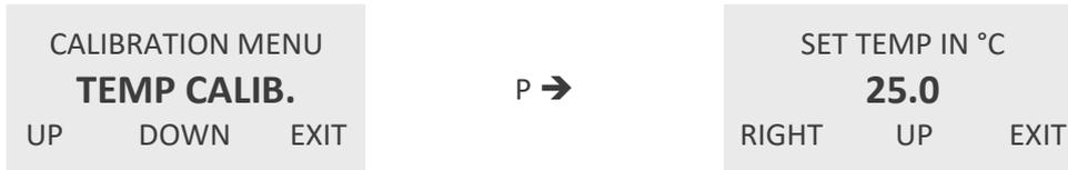
Use the keys "RIGHT" and "UP" to set the actual medium temperature and confirm with "P" or skip with "EXIT". The display returns to the "SERVICE - CALIBRATION" menu.
