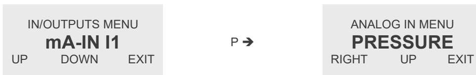
Use the keys “UP” and “DOWN” to select “OFF” or “PRESSURE” and confirm with “P” or skip with “EXIT”.
