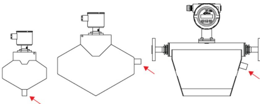
Fig. 3: Rupture disc locations vary by the meter size and style
