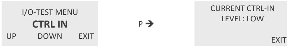
The display shows the actual level at the input. It is automatically updated when the level at the input has changed.
