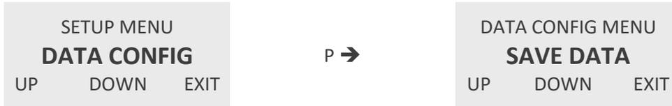
Use the keys “UP” and “DOWN” to select the desired submenu and confirm with “P” or skip with “EXIT”.
