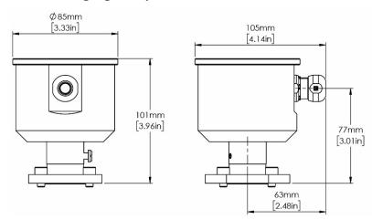
Fig. 42: Dimensions Connection head
