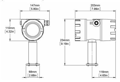
Fig. 41: Dimensions Meter-Mount Transmitter TCE 8000/8100 High Temperature
