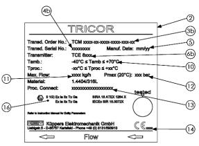
Fig. 15: Device marking TCM remote version
