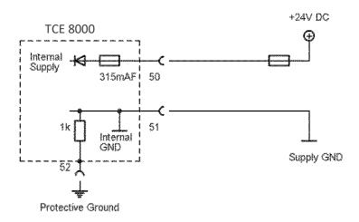
Fig. 20: Wiring diagram for power connections, DC operation
