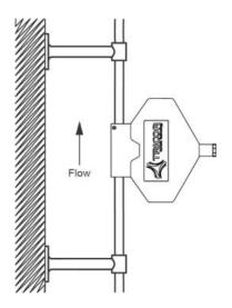
Fig. 17: Vertical Installation
