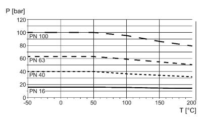
Fig. 29: Metric flange ratings, EN 1092-1 (previously DIN 2628, DIN 2635, DIN 2636, DIN 2637, DIN 2638) (P: Process pressure; T: Process temperature)
