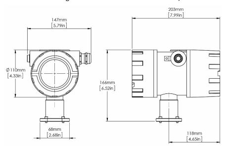
Fig. 37: Dimensions compact transmitter TCE 8000/8100
