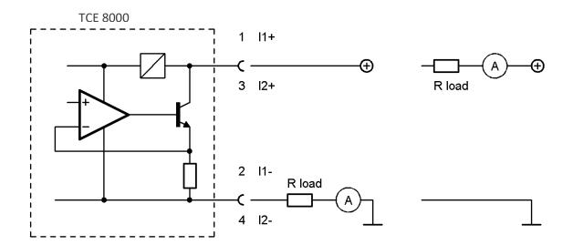
Fig. 23: Wiring diagram for 4 ... 20 mA current loop
