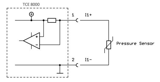
Fig. 24: Wiring diagram for 4  $\dots$  20 mA current input
