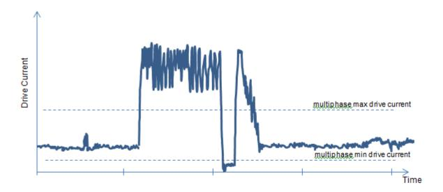
As long as the current drive current stays within the valid range, the flowrate and density will be calculated based on the analog inputs. Otherwise the input signals will be suppressed and the process parameter flow rate and density are set to 0 g/s and 0.001 g/cc.
