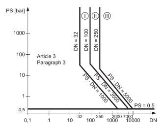
Fig. 26: Diagram 1 for gases of fluid group 2
