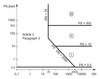
Fig. 27: Diagram 2 for gases of fluid group 1
