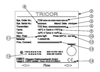
Fig. 14: Device marking TCM compact version
