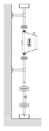
Fig. 18: Installation in a Drop Line
