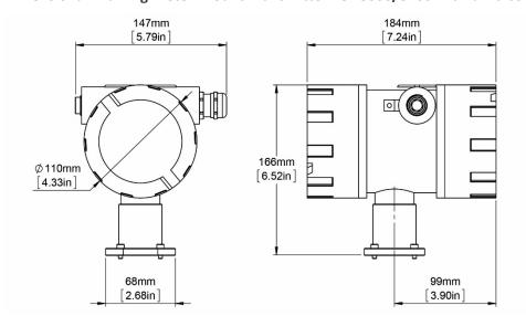
Fig. 40: Dimensions Meter-Mount Transmitter TCE 8000/8100 with blind cover
