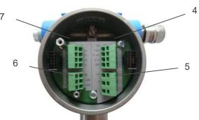
Fig. 12: Electrical terminals TCE 8\*\*\*-W-\*-Ex
