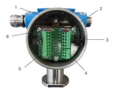
Fig. 11: Electrical terminals TCE 8\*\*\*-W and compact version
