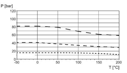
Fig. 30: ANSI flange ratings, ASME B16.5 (P: Process pressure; T: Process temperature)
