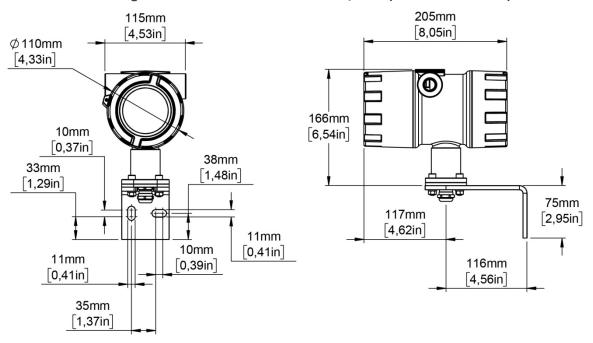
Fig. 39: Dimensions Wall-Mount Transmitter TCE 8000/8100 (for hazardous area)
