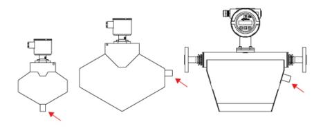
Fig. 3: Rupture disc locations vary by the meter size and style
