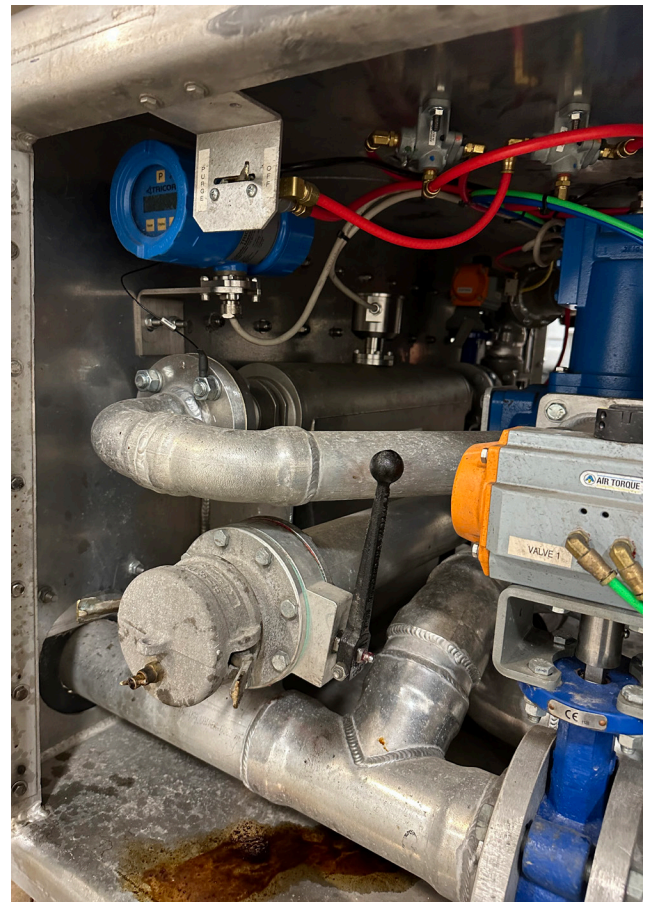
Truck-mounted TCM-65K Coriolis meter
