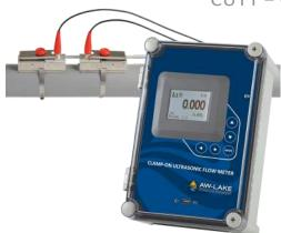
The CUTT Clamp-On Ultrasonic Flow Meter securely attaches to the exterior of metal, concrete, and plastic pipes. The NEMA4X polycarbonate enclosure allows for installation in challenging environments. These non-invasive clamp-on sensors provide advanced flow measurement capabilities without causing pressure drop, making them suitable for diverse applications, including food processing plants, chemical facilities, oil refineries, and more.
